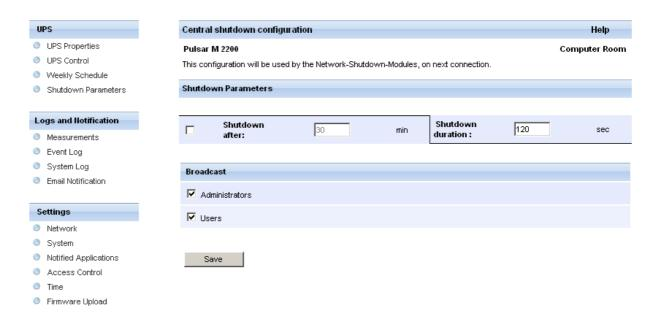
This page is used to define either the "shutdown" or the "notification" settings used by the Network Shutdown Modules that connect to Network Management Card. These settings are used by the Network Shutdown Modules if they are in central-configuration mode or if their configuration is not valid.
